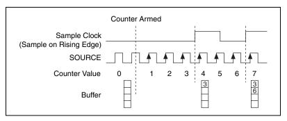
Figure 7-4. Buffered (Sample Clock) Edge Counting
